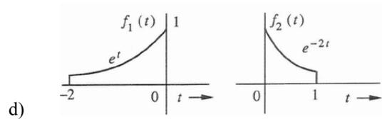
7.\*\*\* Find and sketch  $c(t) = f(t) * g(t)$  for the pairs of functions shown below.
